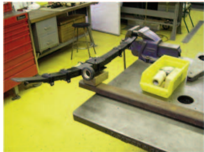
Fig 1 A simple set-up for securing a spring.
